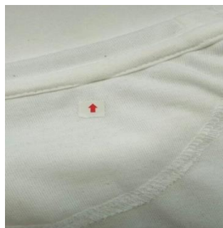
Fig. 5.6: Broken stitch through lockstitch machine
