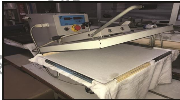
Fig. 3.5: Discontinuous (flat-bed) fusing press
