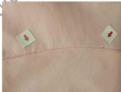
Fig. 5.5: Skipped stitch or broken stitch
