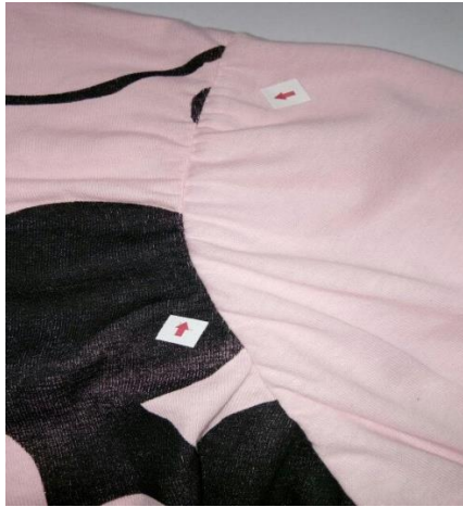
Fig.5.7: upper side view of puckered stitch
